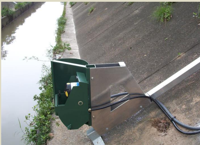
A side-looking (SL) acoustic Doppler velocity meter (ADVM) mounted on a concrete bank provides accurate data on water velocity and level from a position that makes it easy to access and maintain.
