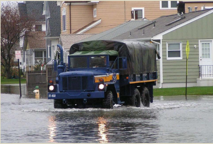
One of two converted surplus military cargo trucks used for high-water responses
