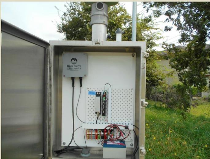
Figure 2 – The ALERT2 back mounted configuration allows easy access to all components, reducing on site maintenance time.
