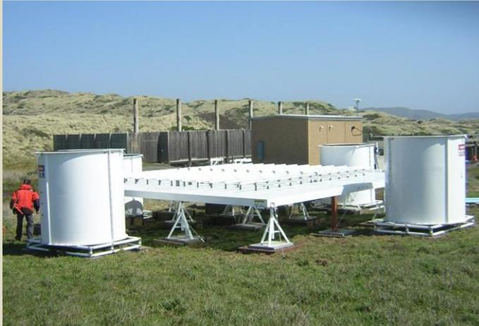
Figure 3. Picture of the Bodega Bay wind profiler as part of the Bodega Bay Atmospheric River Observatory. Photo by Clark King, NOAA ESRL.
