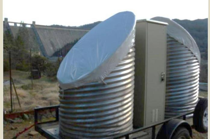
Figure 4. Snow Level Radar at Shasta Dam. Photo by Clark King, NOAA ESRL.
