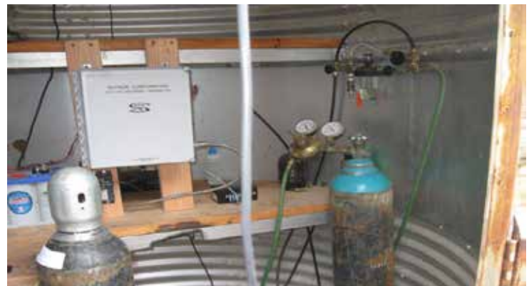
Figure 4b - Old style bubbler with air cylinders
