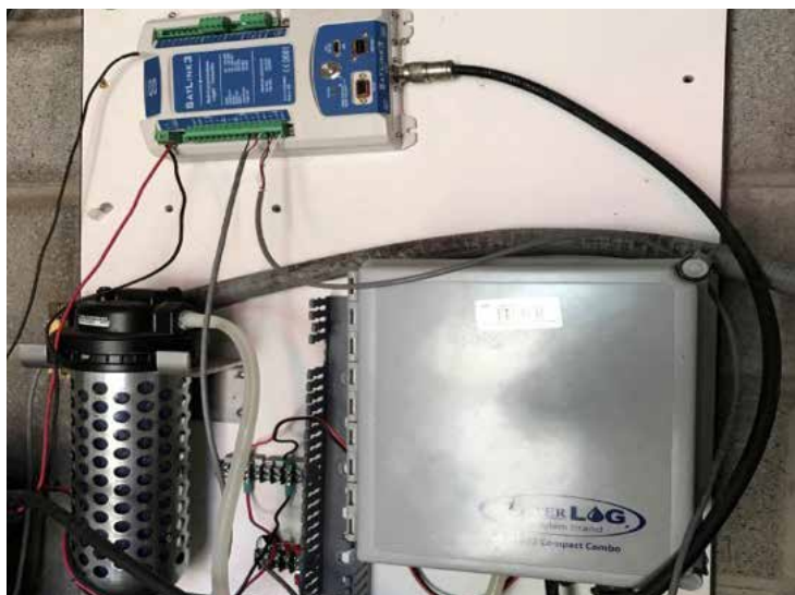
Figure 4c - New-style self-contained bubbler with built-in pump and air chamber
