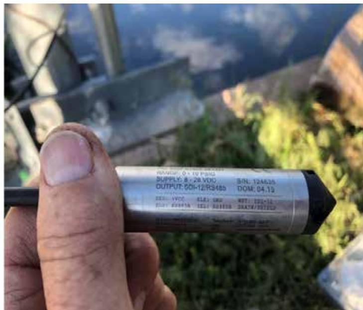
Figure 3a - A vented pressure transducer
