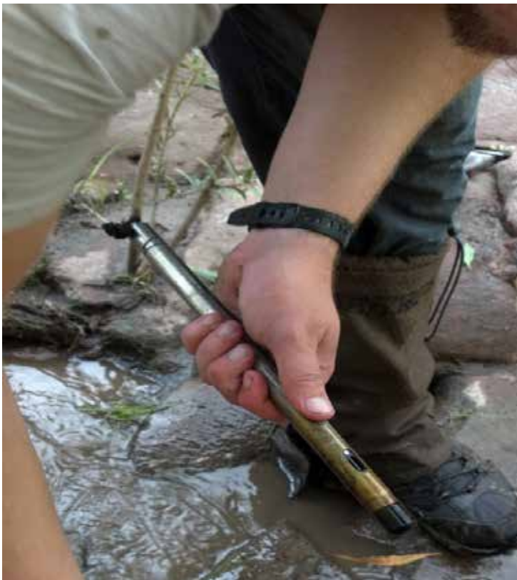
Figure 3b - A non-vented pressure transducer without submersible signal cable
