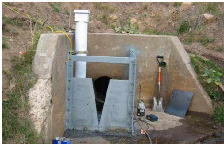
Figure 2c - A float gauge with stilling well at a dam seepage monitoring station – Black Canyon Dam, Arizona
