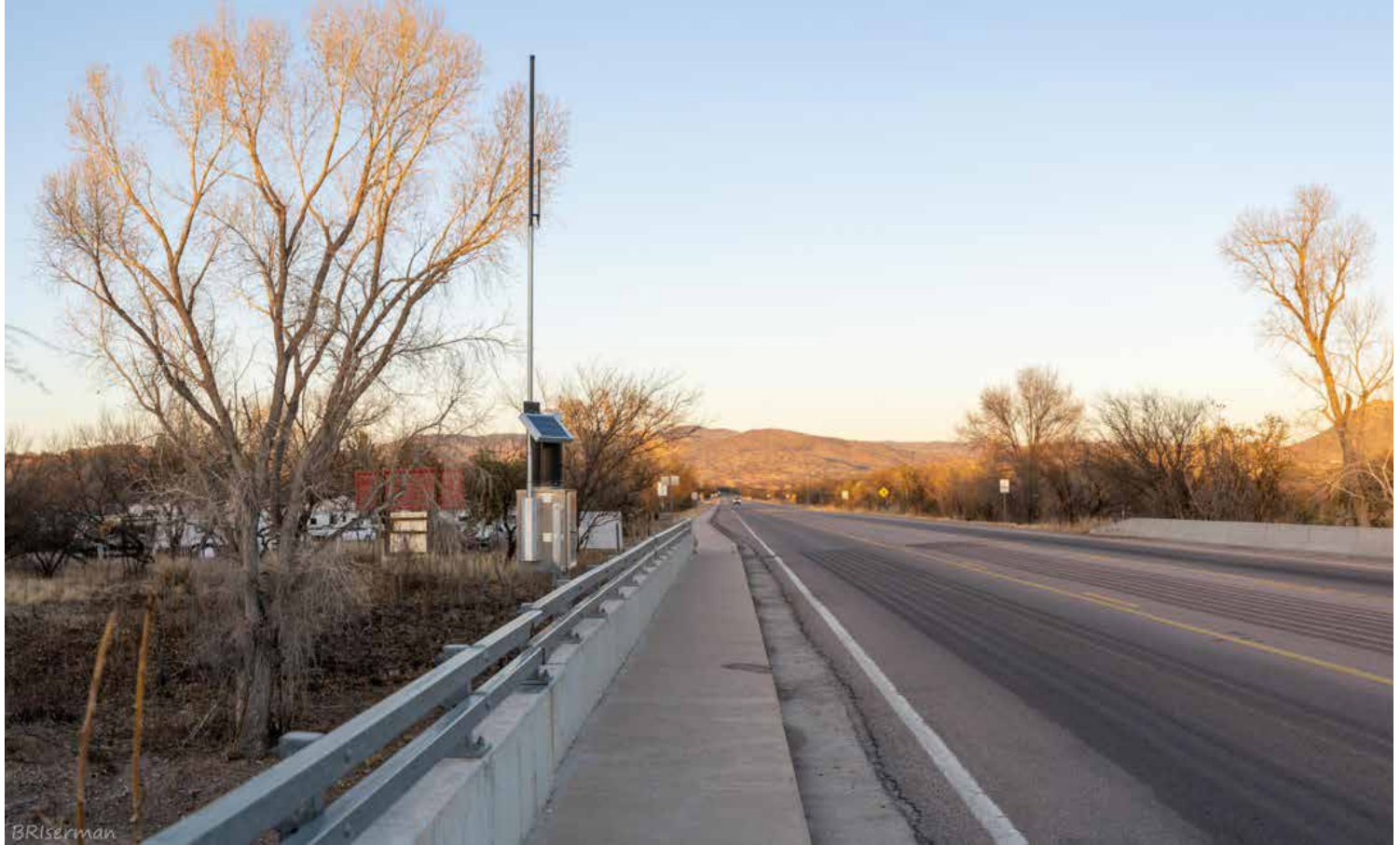
Figure 1 - Streamgauge sited on the “safe side” of the bridge with access via sidewalk
